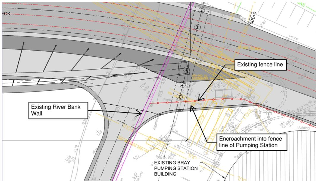
An electrical building which services the pumping station presents a pinch-point in the alignment. It is not possible to provide access past this structure without impacting significantly on the shared path at this location. This building will be relocated to allow for functional passage in his location.
