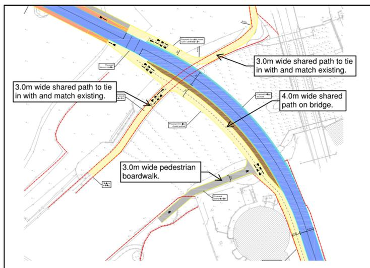
Due to constraints through the southern corridor, a 3.5m wide shared pedestrian/cycleway passage is proposed. The combined footway/cycleway is required to extend connectivity through this corridor and prevent the carriageway from encroaching into the rail boundary. This access then links in with the junction as shown on the figure below.
