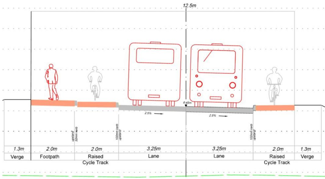
Figure 7 defines the typical alignment cross section between CH 0+200.000m and CH 0+300.000m. This depicts the cross section through the bridge, which includes a 2.0m structural zone to accommodate a central barrier and the support for the cables, which hang from the arch structure to support the deck.
