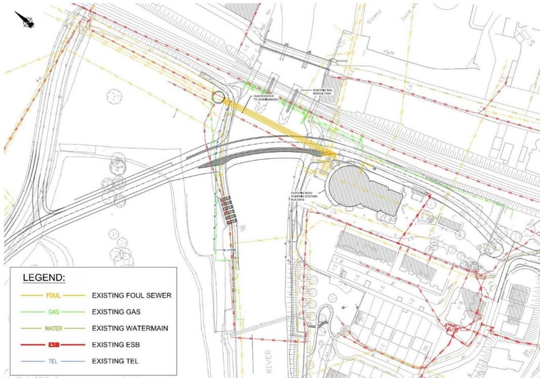
A host of services run parallel to the northern bank, comprising foul, ESB, gas and telecoms. These services will be impacted by the bridge foundations on this bank and will require diversion. Details of this will form part of the utilities relocation package. It is not feasible to avoid the services on this bank without substantially increasing the span of the bridge.
