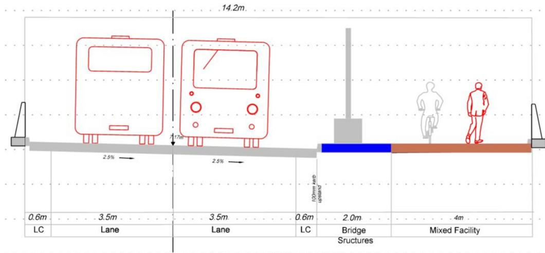
Figure 8 defines the alignment cross section between CH 0+300.000m and CH 0+457.900m to where the link road ties in to the junction at Seapoint Road. This narrower configuration is due to the boundary constraints caused by the railway line and Bray Pumping Station.
