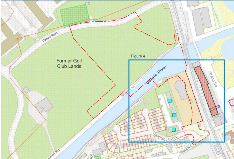
To the south, the proposed link road alignment is highly constrained by Bray Pumping Station and the railway boundary. A Gas Networks Ireland site is also located to the south, adjacent the junction with Seapoint Road. These boundary constraints create a confined corridor through which the proposed link road must pass, impacting on the available space to accommodate both pedestrian and cycle paths alongside the proposed carriageway.
